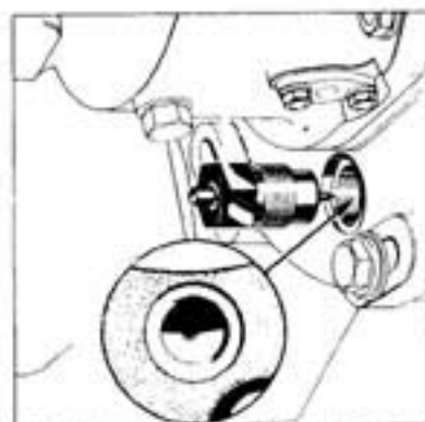
FIG. 10 INJECTION PUMP TIMING TOOL
